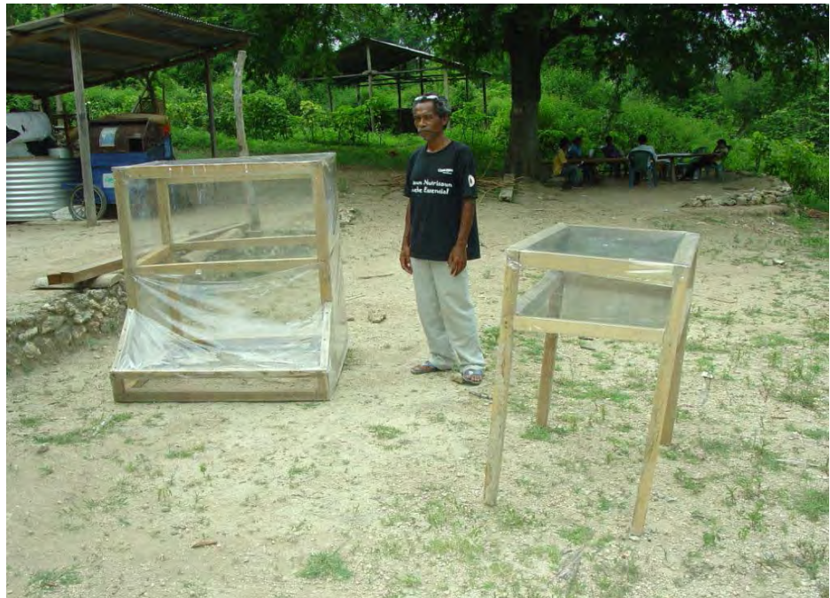
A man shows the two parts of a solar dryer that when put together are used to dry out vegetables, Ra'ano, February 2010.
